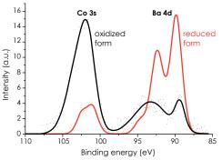
A catalyst sample - carbon sample coated with cobalt oxide  ${\rm Co_3O_4}$  and barium carbonate  ${\rm BaCO_3}$ , was examined just after impregnation. Co 3s and Ba 4d XPS spectra were obtained: black line marked as oxidized form of the catalyst. XPS analysis shows a considerable share of cobalt in the surface layer (in the form of oxide). There are only few barium compounds in this layer.
