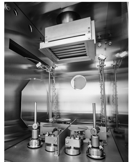
View into the vacuum chamber Chamber floor: Three thermal single evaporators. Chamber ceiling: substrate stage with gradient aperture and two thickness gauges.
