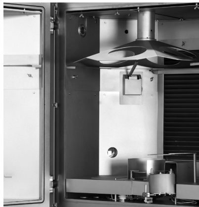
Substrate calotte rotating on the chamber ceiling with central measurement of the layer thickness based on oscillating quartz. Chamber bottom: Electron beam evaporator with multi-changing crucible and ion source.
