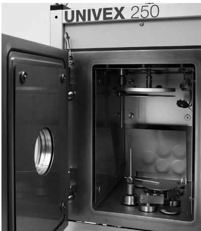
Chamber bottom: double thermal evaporator with source shutter Chamber top: rotating substrate table with substrate shutter
