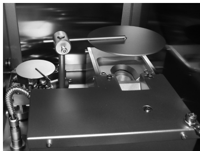
Electron beam evaporator with fourfold rotating crucible as well as additional double thermal evaporator, each with source shutter
